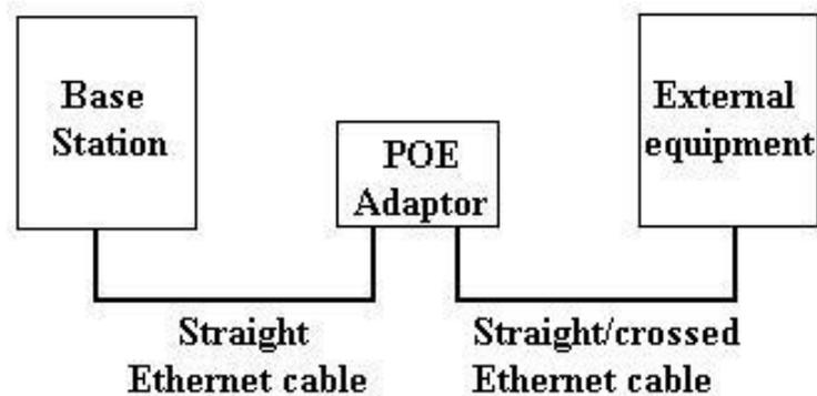
Figure 1 - Hardware setup
